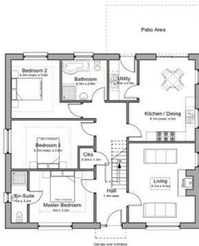
Proposed Ground Floor Plan 113m 2 / 1215 Sq ft. Scale 1:100
